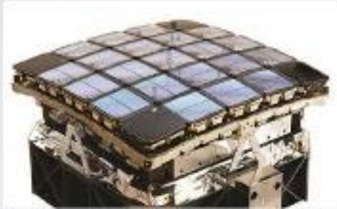
Kepler focal plane, 42 flat CCDs
